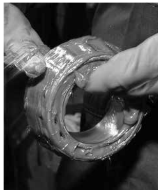
Fig. 147. Grease can easily be packed by hand.
