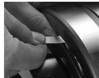
Fig. 95. Measure of RIC before installation.
