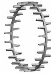
Fig. 45. One-piece, machined-brass, land-riding, finger-type cage.
