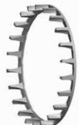
Fig. 46. Split, machined-brass, land-riding, finger-type cage.
