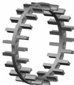
Fig. 49. One-piece finger-type cage.
