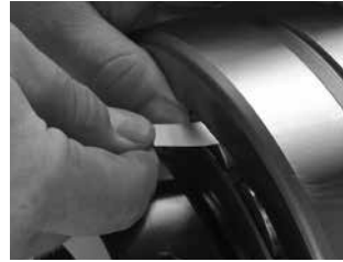
Fig. 91. Measure RIC before installation.
